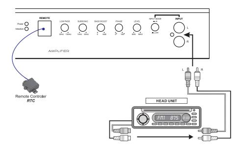
The SERIES amplifier offers RCA-Inputs, which are connected through cinch cables with the preamplifier-outputs of the head unit. IHLAC and RCA III adapter cable can be purchased as accessories if the head unit has no RCA output.
